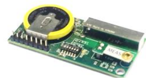
Fig.7 - A wireless sensor powered by a CR2450 battery
