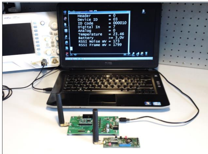
Fig. 3 – Transmit and receive messages with the "Basic" Demo Kit
